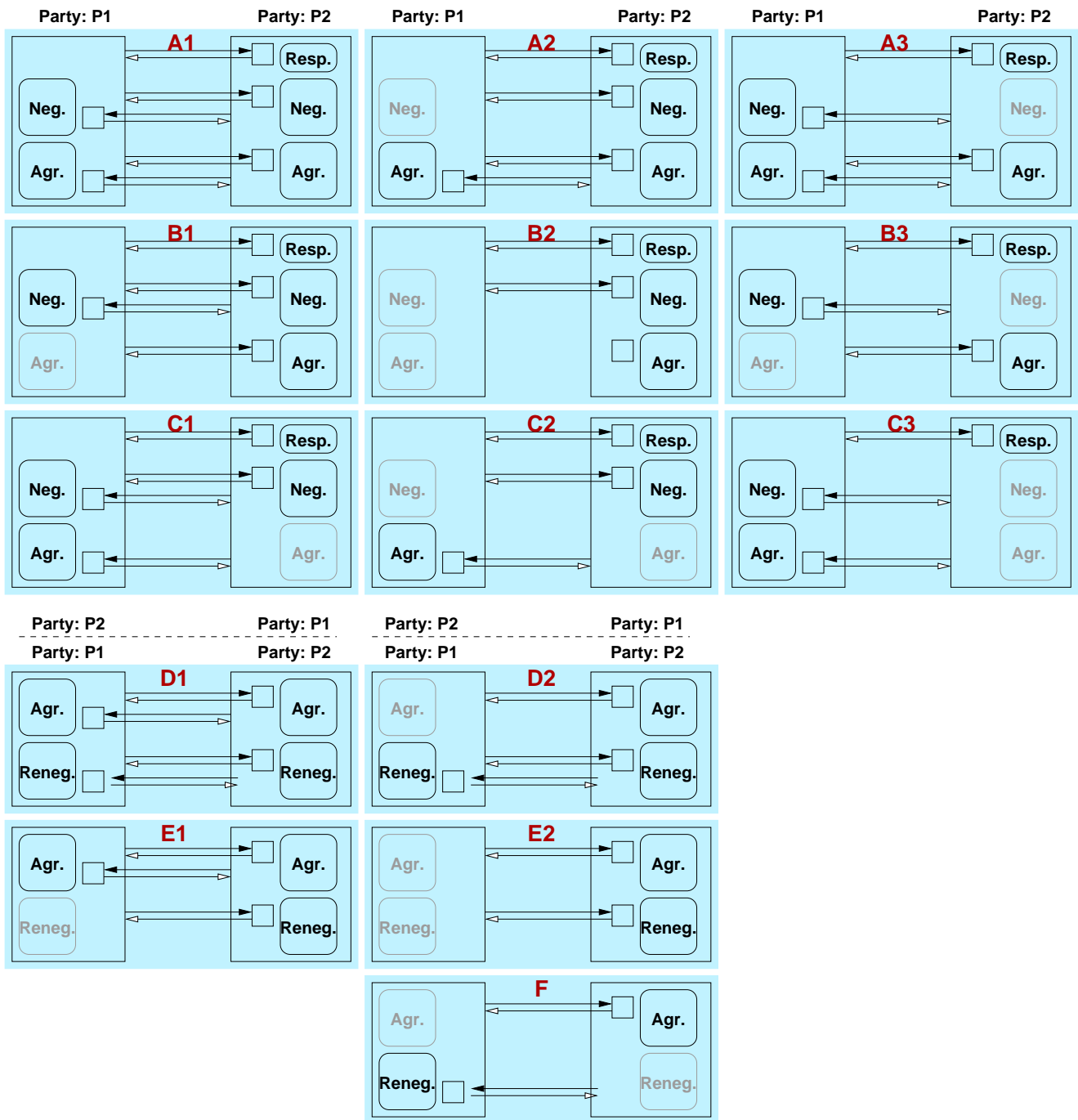
Figure 5. Full range of possible asymmetric combinations. Asymmetry is not limited to pure client-server but can also surface through role-reversal , where the initiating party becomes the main contact point for further messages. Negotiation and Renegotiation asymmetry can be considered separately, with the impact of Negotiation resulting in symmetric or asymmetric Agreement between the phases. Four Renegotiation asymmetry scenarios are omitted because they are equivalent to one of the existing ones, but with the party names reversed.
