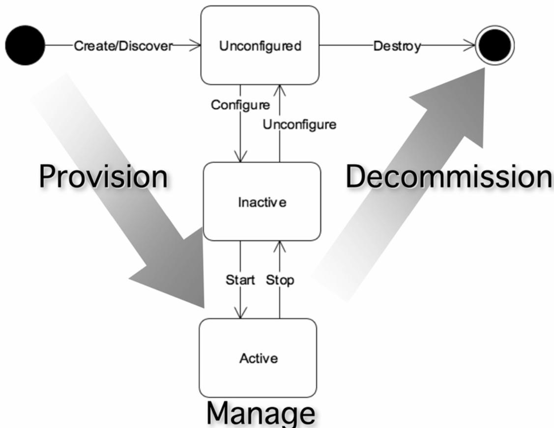
Figure iii – The General Grid Component Life Cycle
